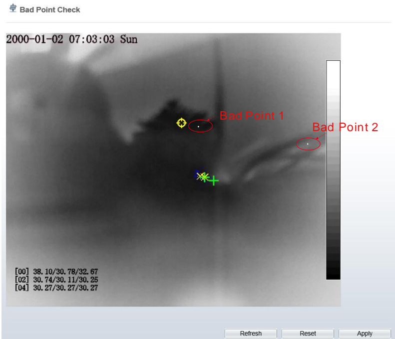
Figure 4-12 Bad Point Check
